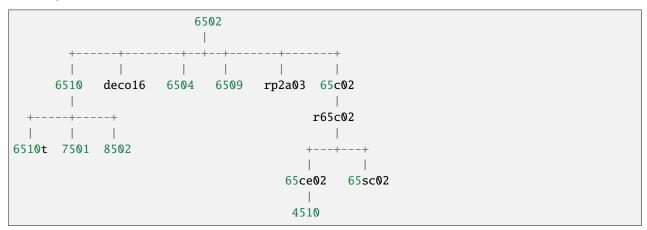
The 6510 adds an up to 8 bits I/O port, with the 6510t, 7501 and 8502 being software-identical variants with different pin count (hence I/O count), die process (NMOS, HNMOS, etc.) and clock support.
